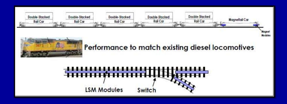
Half a mile track testing including switching and multiple vehicles under typical port operating conditions
