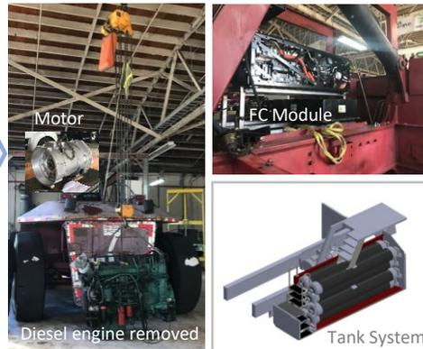
FC Module=Phase 1 & 2, Tank and components = Phase 2 (plan)
