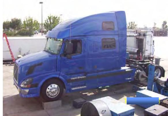
**Figure 1. HD Truck on Chassis Dynamometer**
