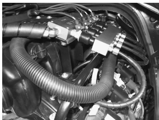
Figure 12: Baytech's CNG Injector Block Installed on GM 6.0L Van
