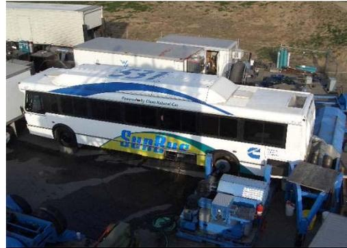
Figure 1 Transit bus on WVU Transportable Heavy-duty Chassis Dynamometer
