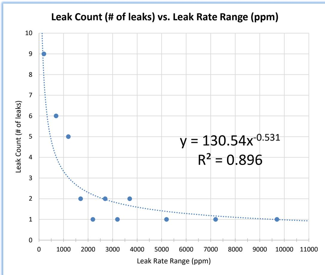
These curves and power trendlines are able to predict, with relatively high confidence, the number of additional leaks estimated above a leak standard at differing leak values:
