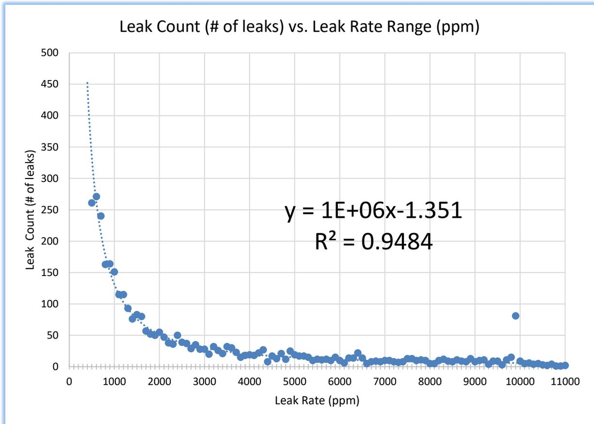
**Figure 2-4 Distribution of Pump (Light Liquid), Compressor Leaks**
