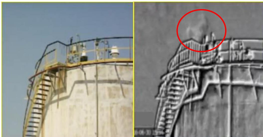
Figure 2-1: View with naked eye compared to view with an OGI camera
