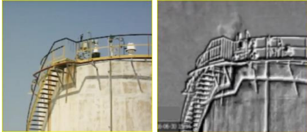
Figure 2-1: View with naked eye compared to view with an OGI camera
