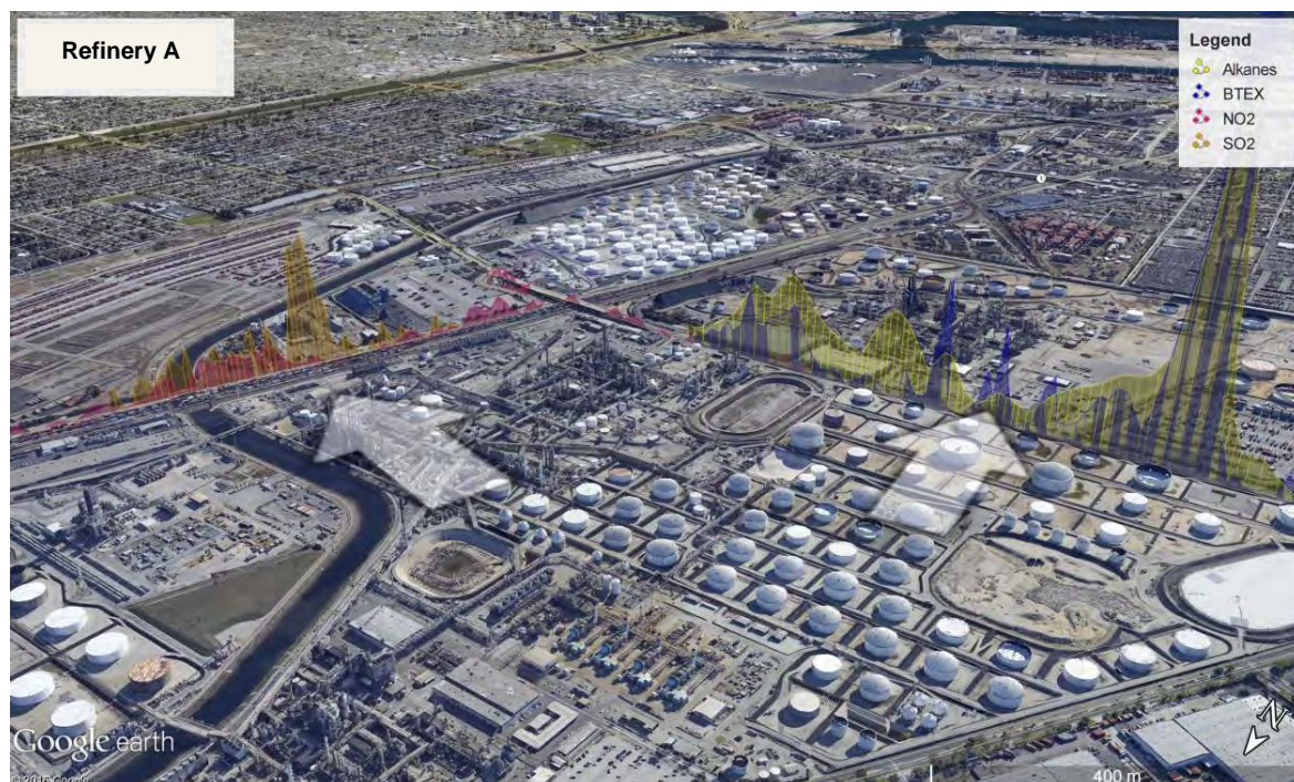
Figure 21. Transects of plumes originating from Refinery A. NO 2 (pink line) and SO 2 (brown line) were impacted by westerly winds. Conversely, BTEX (blue line) and alkane (yellow line) plumes were measured in the presence of northerly winds. The column thickness for both NO 2 and SO 2 is reported on the same scale (max NO 2 = 3 mg/m 2 flux NO 2 = 114 kg/h, max SO 2 = 11 mg/m 2 flux SO 2 = 46 kg/h). Alkanes and BTEX columns are scaled separately for better visibility (max BTEX = 0.25 mg/m 3 , max alkanes = 1.95 mg/m 3 ). The examples presented here are single transects made on September 2 and on September 19, 2015.
