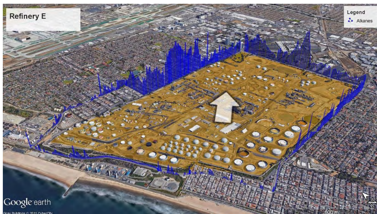
Figure 42. Example of a SOF ‘box’ measurement of Refinery E (orange area) 6 November 2015, 10:47-11:22. Alkane column is shown as a blue curve with apparent height proportional to gas column (10 m equivalent to 1 mg/m 2 , max 55 mg/m 2 ). Wind direction during the measurement is indicated by the white arrow. Average wind speed during this particular measurement was 1.8 m/s. Emissions on the upwind side are subtracted from the downwind side in order to get emissions from within the box. This particular transect measured 229 kg/h from Refinery E.
