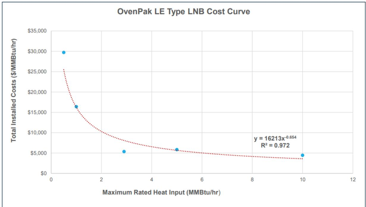
Figure 2-6. OvenPak Type LNB Burner Cost Curve
