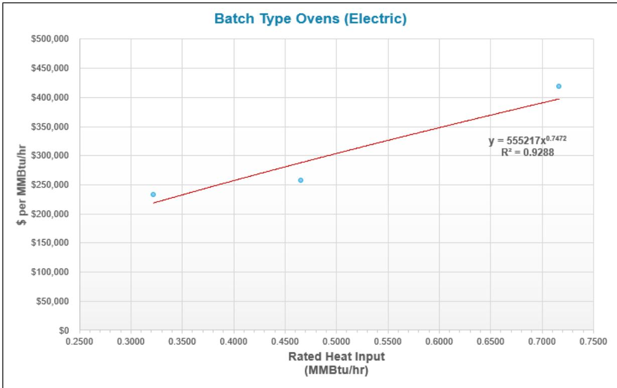
Figure 2-8. Electric Batch Oven Cost Curve
