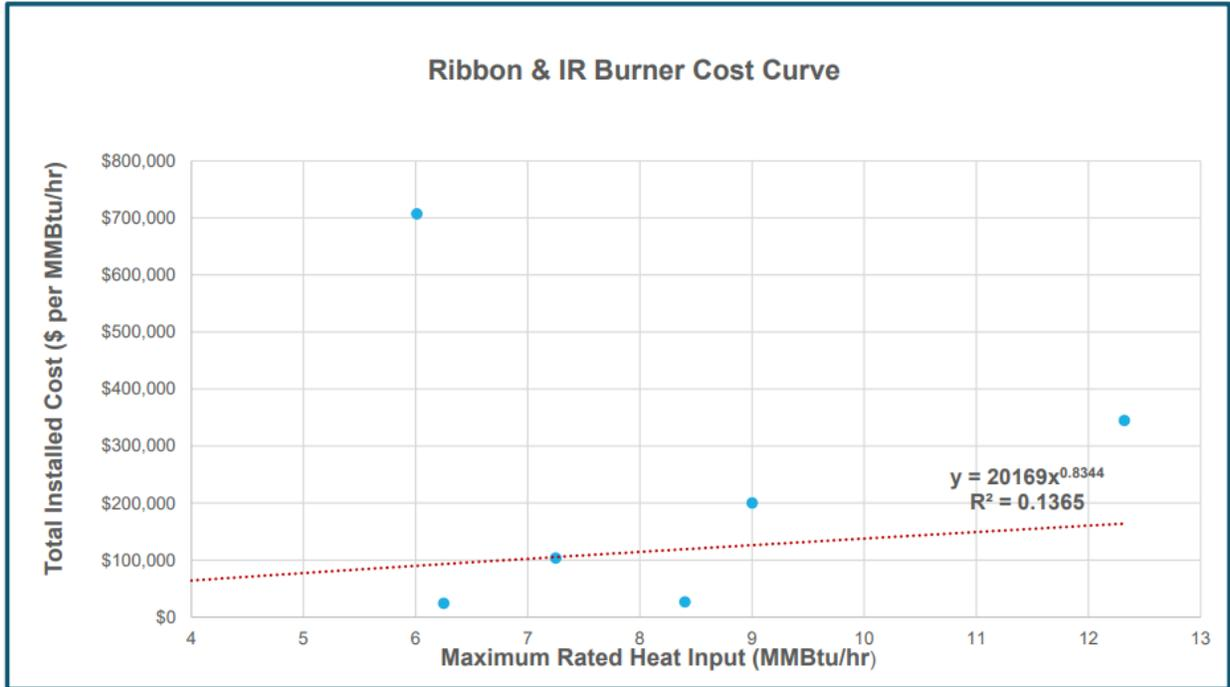
Figure 2-5. Ribbon and IR Burner Cost Curve
