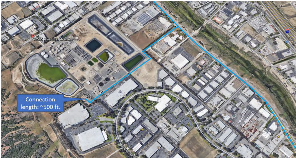
Figure I.3: TVRWRF Pipeline Connection
