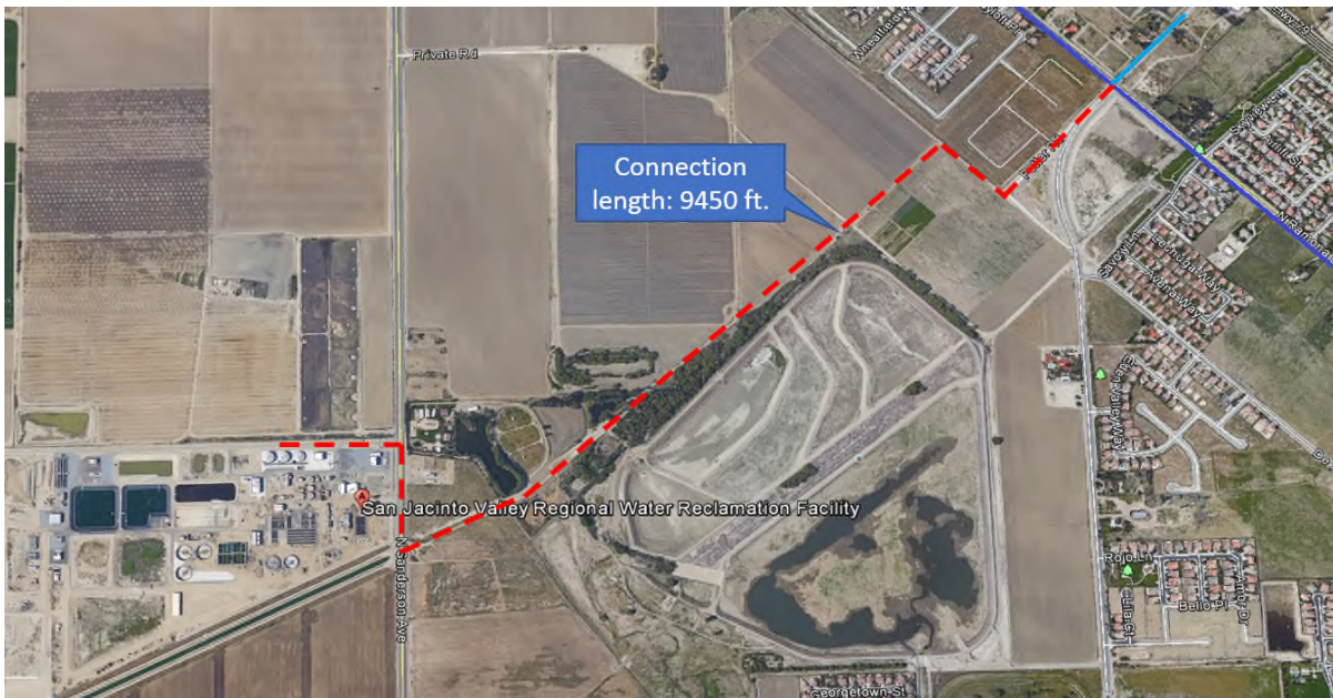
Figure I.4: SJVRWF Pipeline Connection
