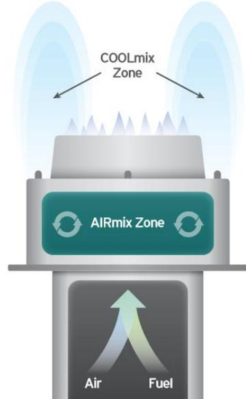
*The SOLEX burner achieves 5 ppm NOx and near-zero CO at start-up, all with a short flame length.*
