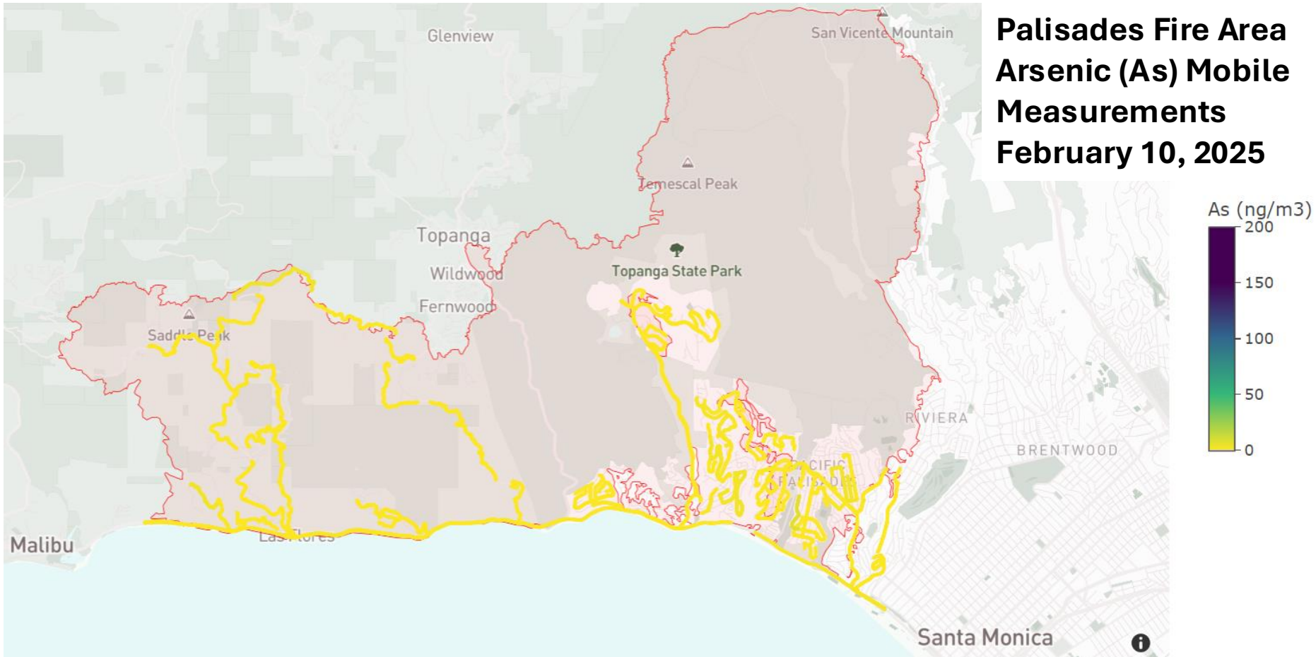
Figure 12. Map shows concentrations of Arsenic (As) measured on February 10, 2025. Results were well below the state's short-term (1-hour) health threshold for this pollutant (200 ng/m 3 ).
