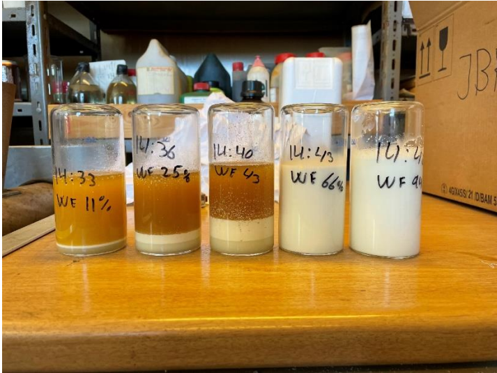
Figure 5 – Unstable emulsions vs stable
