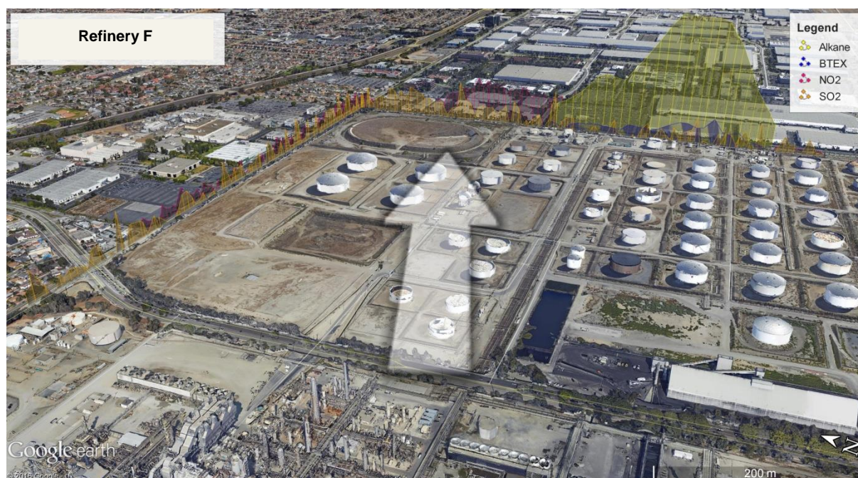
Figure 51. Transects of plumes originating from Refinery F: NO_2 (pink), SO_2 (brown), BTEX (blue) and alkane (yellow). NO_2 and SO_2 show column thickness and are both on the same scale (max NO_2 = 5.0 mg/m 2 , flux NO_2 = 38.2 kg/h, max SO_2 = 4.4 mg/m 2 , flux SO_2 = 17 kg/h), alkanes and BTEX show concentrations and are scaled independently for visibility (max BTEX = 0.01 mg/m 3 , max alkanes = 0.55 mg/m 3 ). Example transects from September 17, 1:22 PM and 11:36 PM.
