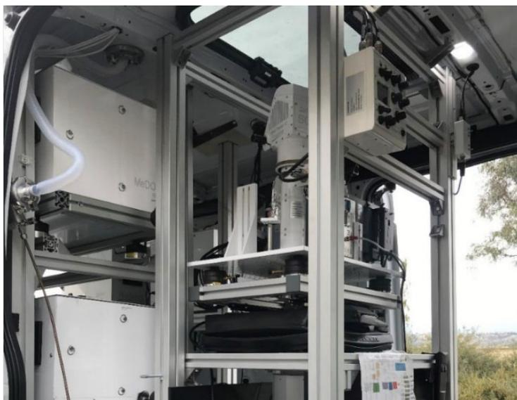
Figure 3. Picture of the solar occultation flux (SOF) instrument mounted inside the ORS ML.
