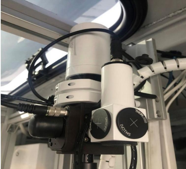
Figure 4. Picture of the SkyDOAS telescope mounted inside the ORS ML.
