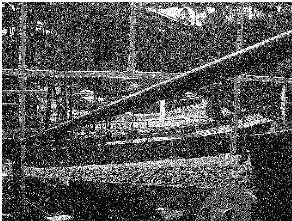
Figure 2. South-side view of sampling array on downwind side of the conveyor transfer point at the Barstow plant.
