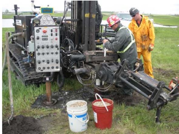
Figure 14- Waste sampling using a Sonic drilling unit
