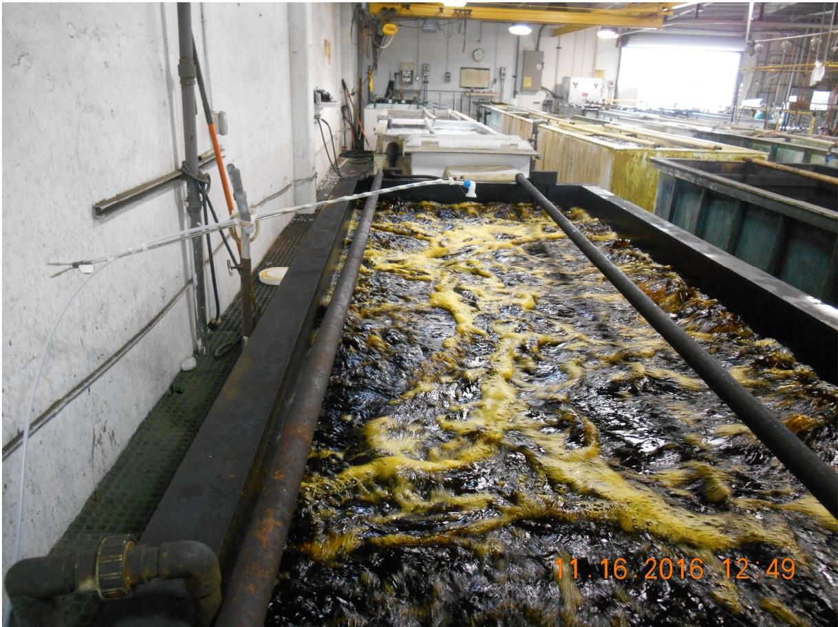
**Figure 2: Air Agitated Chromate Film Tank #43**
