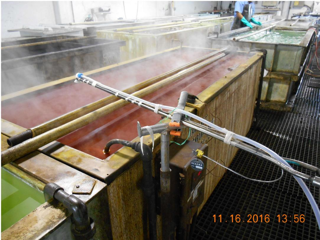
**Figure 1: Heated Dichromate Seal Tank #22**
