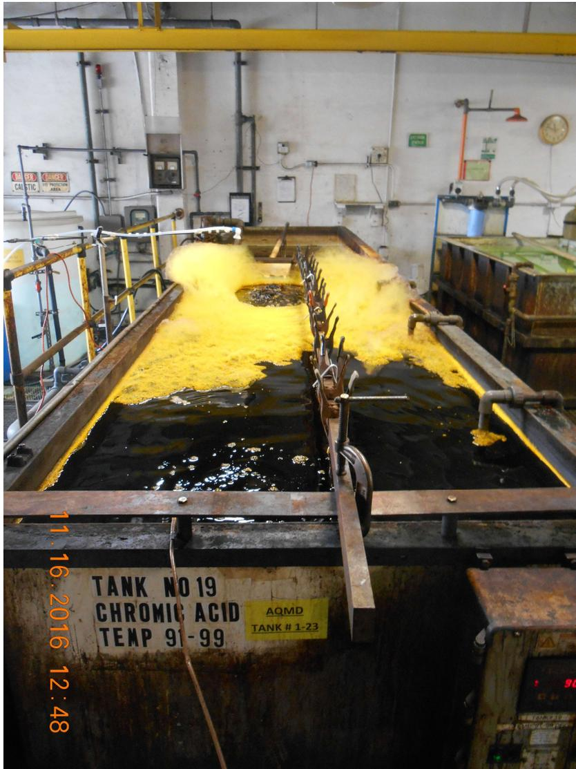
**Figure 3: Air Agitated Chromic Acid Anodizing Tank #19**
