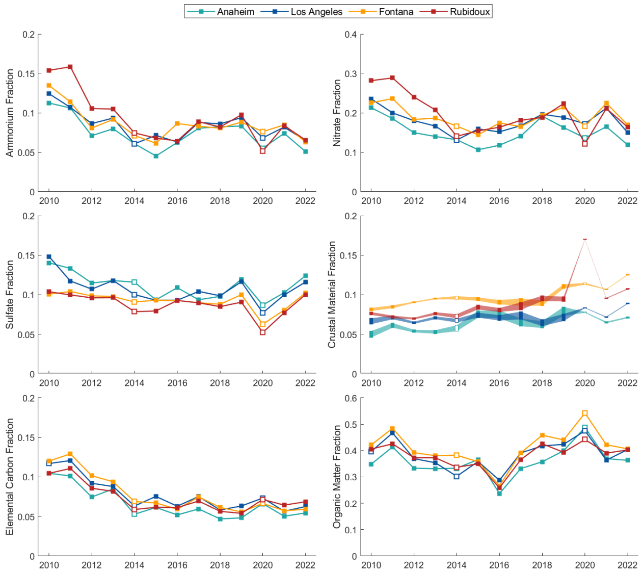
FIGURE 2-15 SOUTH COAST AIR BASIN PM2.5 SPECIATION NETWORK WEIGHTED ANNUAL AVERAGE RELATIVE CONTRIBUTION TRENDS OF RELATIVE CONTRIBUTION TO MASS, 2010–2022 16
