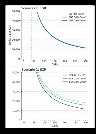
Operational threshold has minimal effect on EGR costs, but a large effect on SCR costs due to changes in catalyst (urea) consumption
