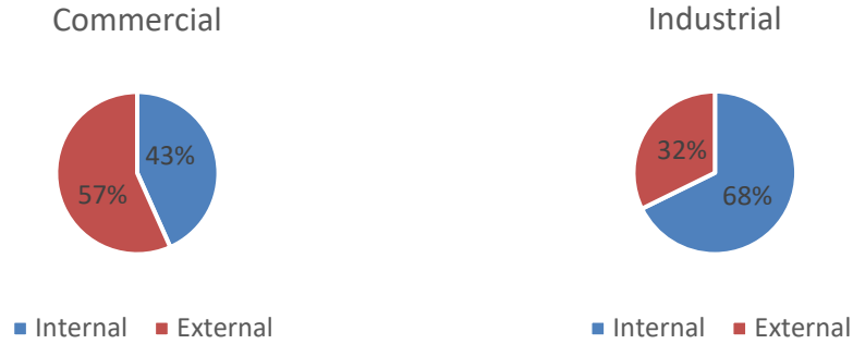
Figure 3. The relative contribution of internal and external combustion in the industrial and commercial sectors as determined from AER throughput data
