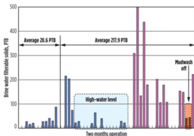
**Fig. 5.** Tank pretreatment impact on desalter filterable solids.
