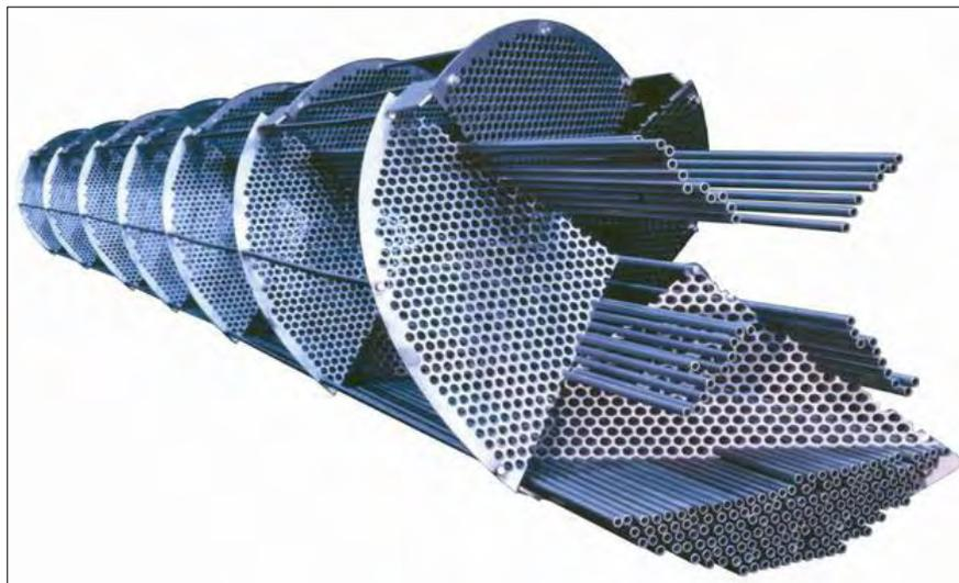
Figure 5 HelixChanger tube bundle in fabrication
