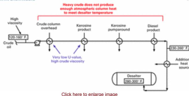
Fig. 5 An alternate approach is adding exchangers in series with existing exchangers (Fig. 5), which minimizes fouling and increases pressure drop. Heavy crude revamps typically require larger charge pump motors and impellers and sometimes pump
