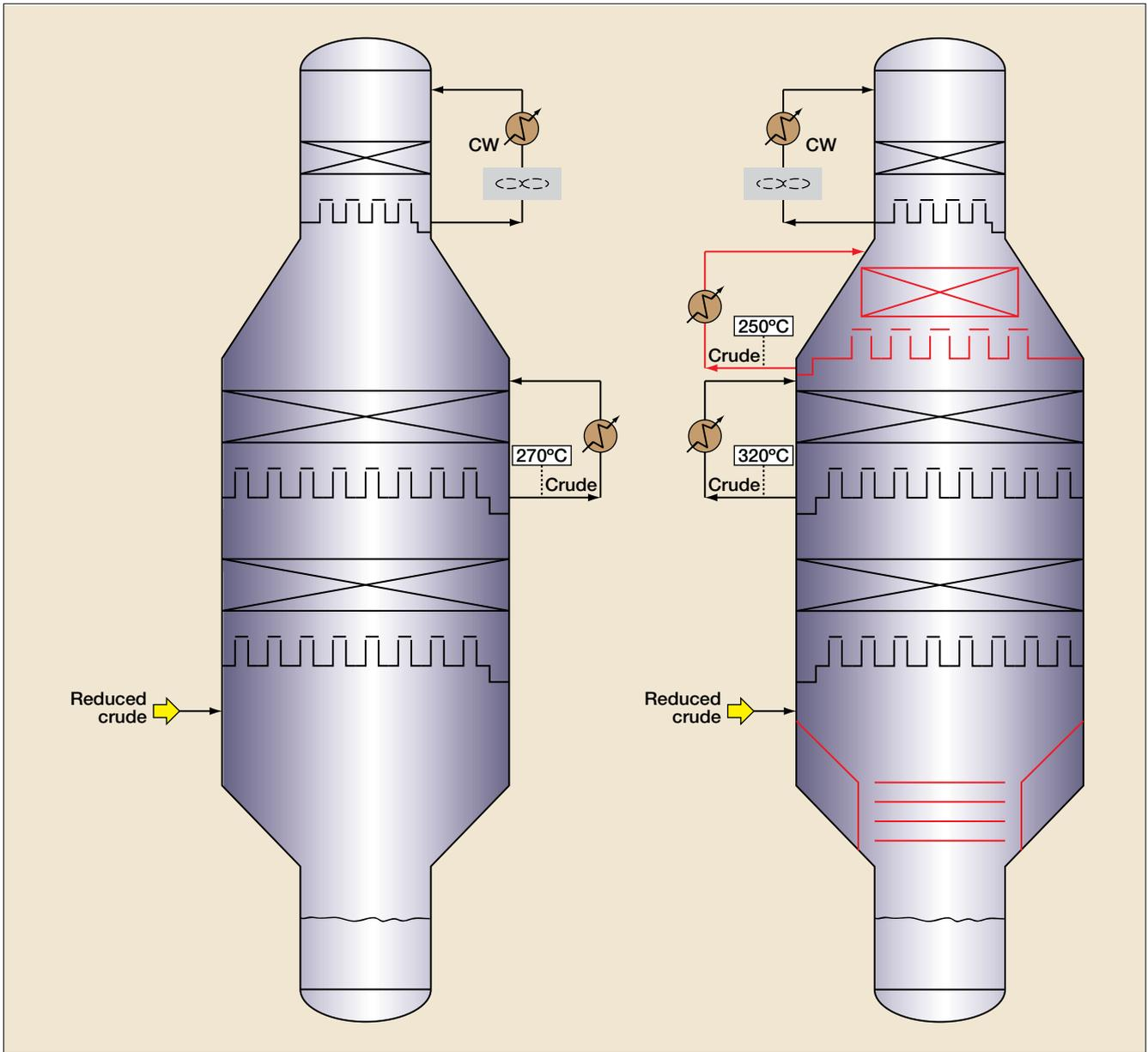
Figure 3 Vacuum tower MVGO pumparound
