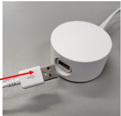
Insert the larger end of the USB cable into the nest power supply
