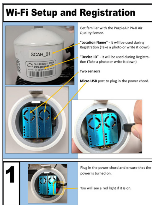
Figure 4-1. Excerpt of PurpleAir PA-II installation instructions produced by the Bay Area Air Quality Management District in collaboration with the Oakland, CA, community partner, Asian Health Services. Less text and more images were used to facilitate translation into seven languages used in the community.
