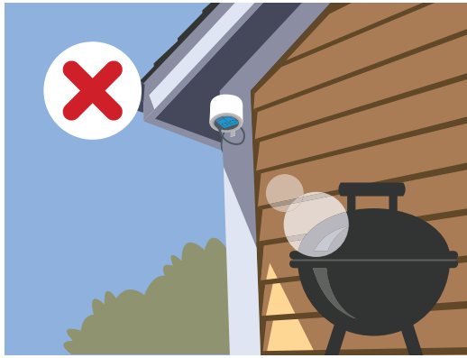
Poor location: The sensor is placed too close to a source of emissions that will affect measurements.
