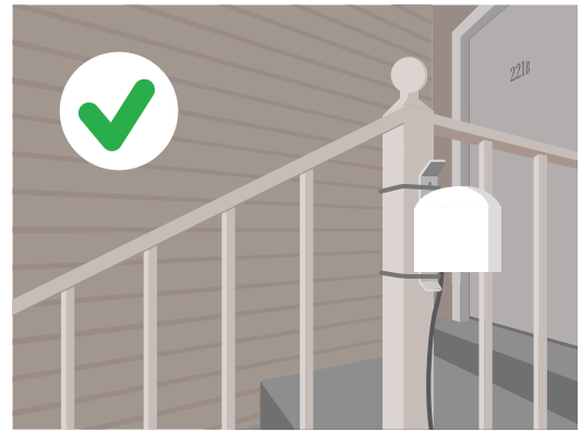
Good location: Breathing height can be higher off the ground, such as outside this second-story apartment.
