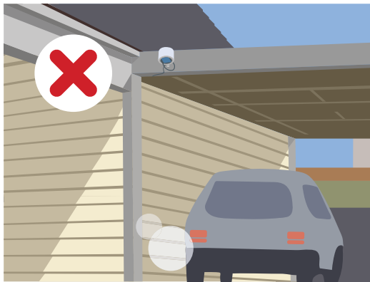
Poor location: Think about how the location will change if, for example, a car is idling near your sensor.
