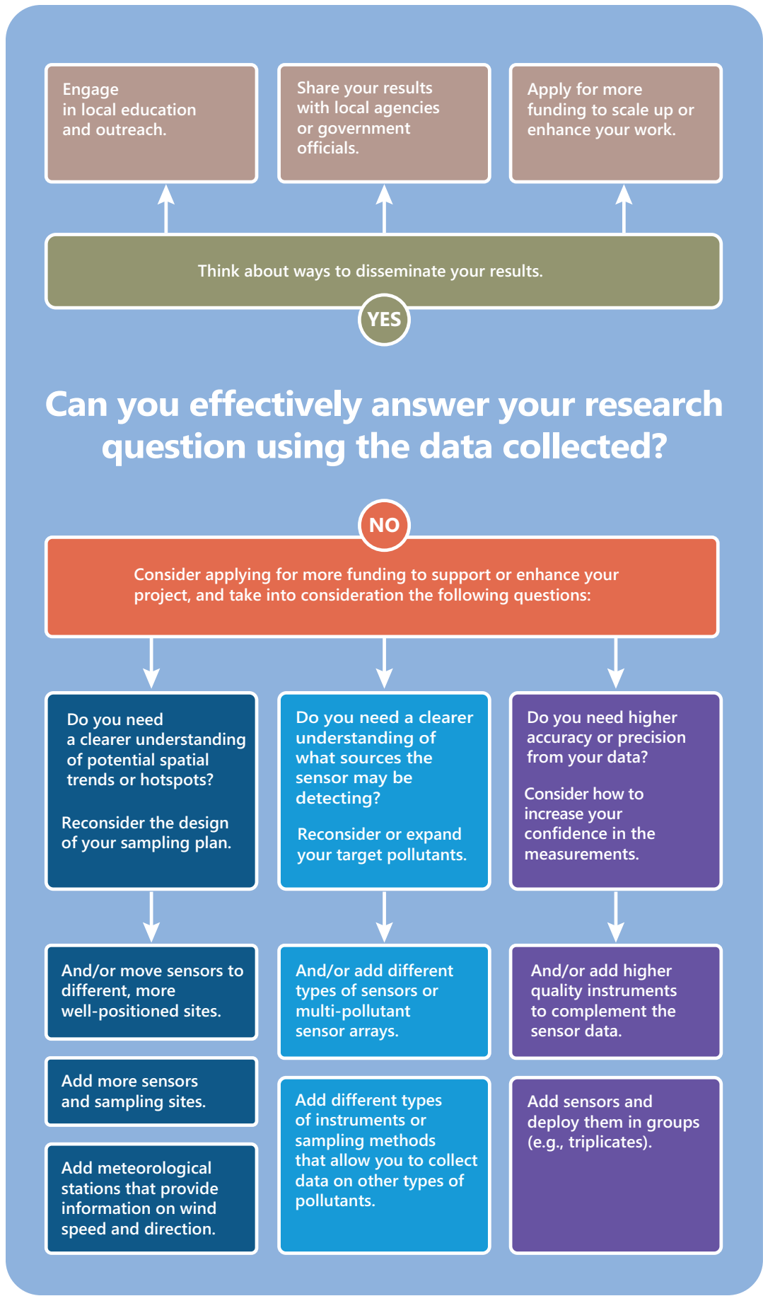
Figure 5-1. Use this decision tree to determine whether more measurements are needed to meet project objectives.
