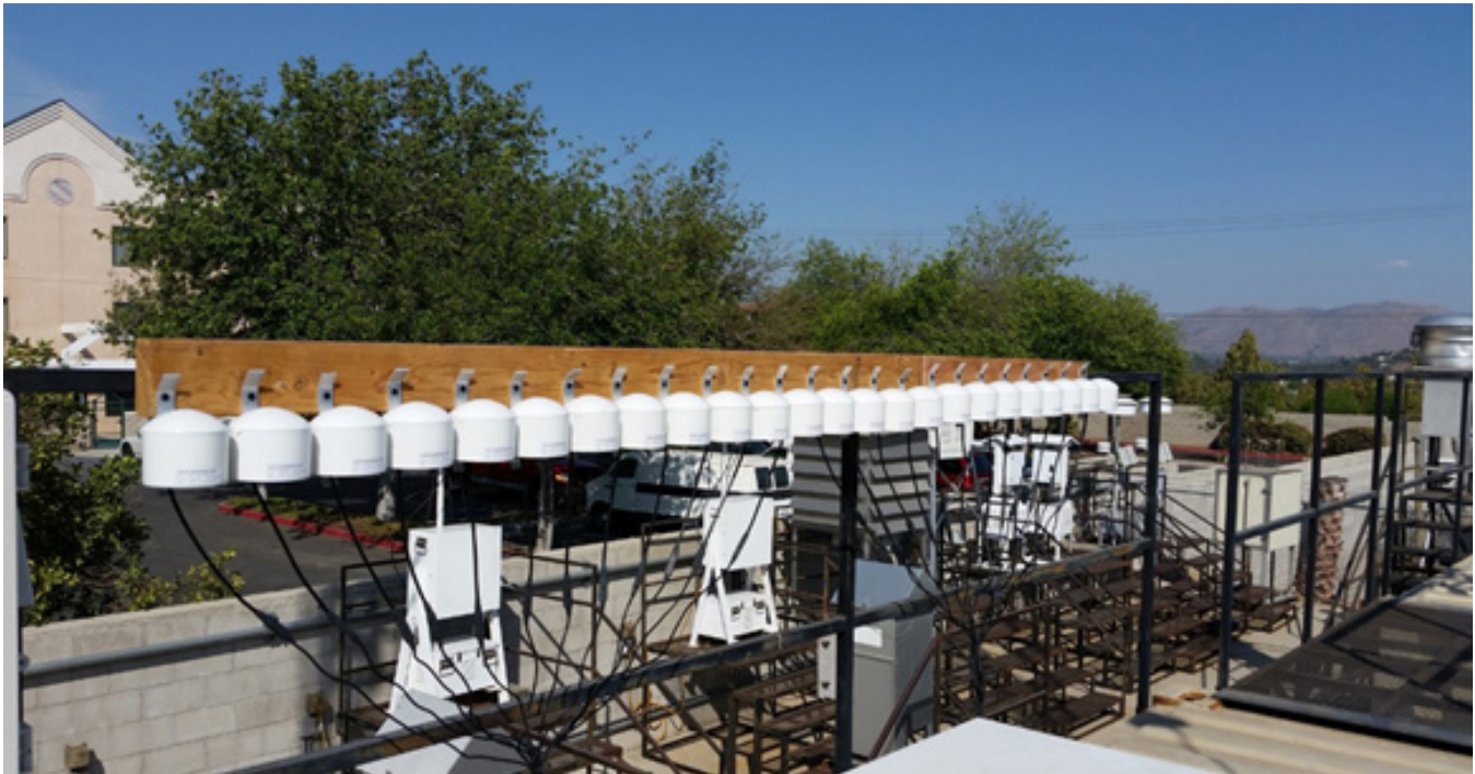
Figure 4-3. PurpleAir PA-II sensors collocated with regulatory monitors at the South Coast AQMD Ambient Monitoring Station site in Rubidoux, California
