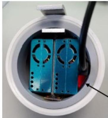
A red LED will be on when the sensor is powered.
