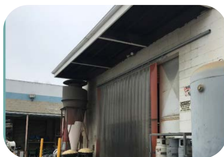
Cross-Draft Minimization Using Overlapping Strip Curtains
