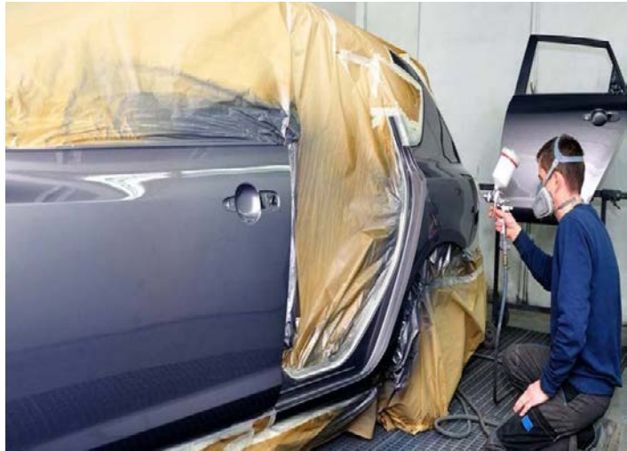
Figure 4-13: Application of Automotive Coating Inside a Paint Spray Booth
