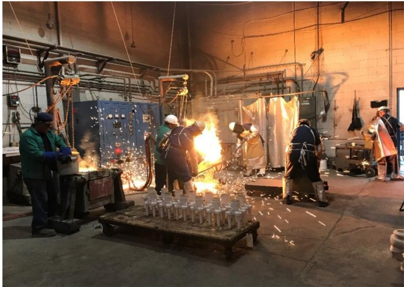
**Figure 4-11: Pouring Molten Metal into Molds**
