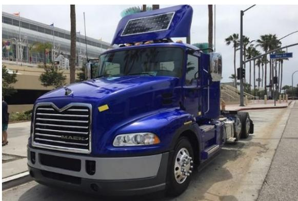
**Figure 7: Volvo Diesel Hybrid Drayage Truck**
