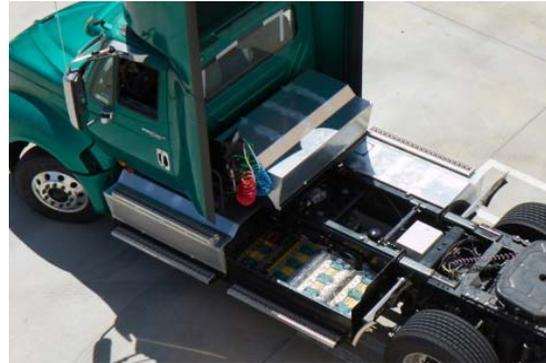
Figure 1: A demonstration vehicle equipped with Inverter-Charger Unit
