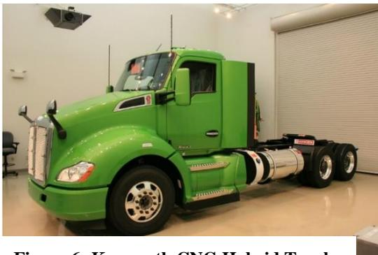
**Figure 6: Kenworth CNG Hybrid Truck**
