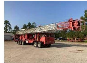
Example of a Workover Rig
