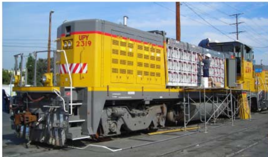
Railpower Green Goat™ having replacement set (25 tons, largest possible package space-wise) of lead-acid batteries installed with stronger assembly rack, impact detectors and improved ventilation system. 265 hp diesel-generator (for recharging batteries) is behind louvers at rear end. (October 30, 2010)
