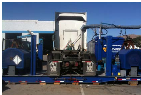
Figure 1: Test Vehicle during chassis dynamometer testing
