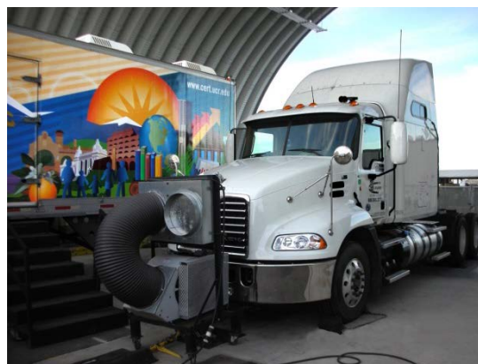
Figure 1: Truck being tested on chassis dynamometer
