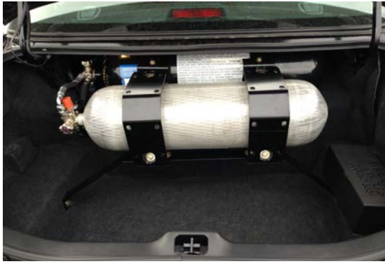
Figure 2: Type 3 CNG Fuel Tank upgrade installed in trunk of PPV; 4.5 GGE of fuel capacity.
