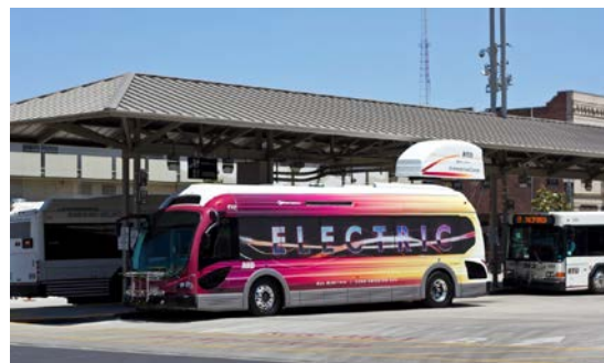
Figure 1: Ecoliner Bus Being Charged at Foothill Transit's Pomona Station
