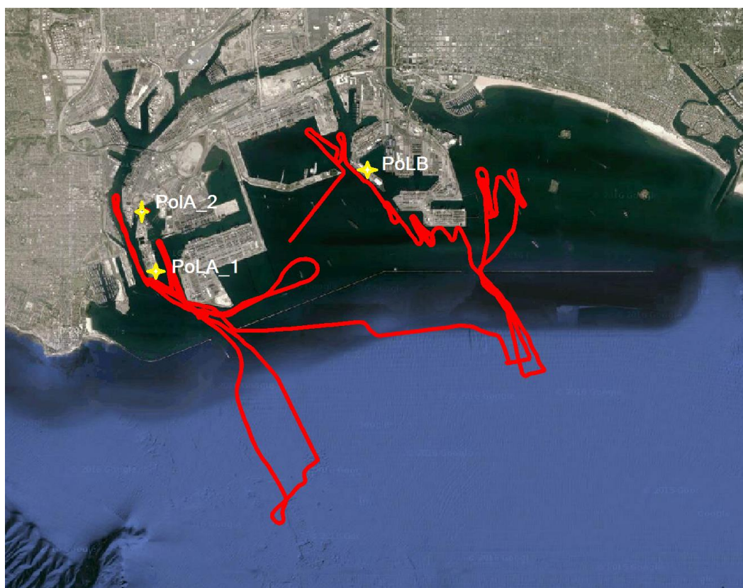
Figure 7. Fixed ship emission measurement sites in Port of Los Angeles and Long beach, respectively, shown by stars, together with a GPS track of the measurement vessel, Yellow Fin for one of the campaign days.
