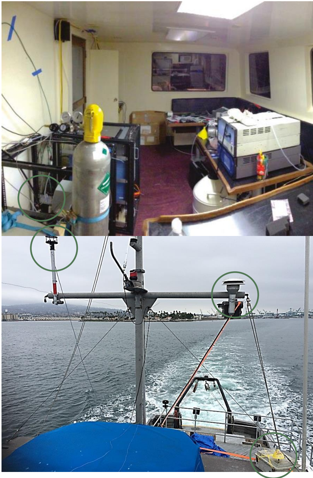
Figure 10. The measurement setup inside the Yellow Fin is shown in the upper picture while the gas and particle inlet system is shown in the lower picture on the right-hand side. Here a particulate matter inlet, typically for PM10 measurements, is here connected to 7 m Teflon tubing for the gas analysis and antistatic tubing for the particle analysis. On the right-hand side in the lower picture is shown a sonic wind meter. On the lower right-hand side in the picture is shown the OPS measuring the fine/coarse particles between 300 nm to 10 \mu\text{m} . Only a short 15 cm tubing was used here.
