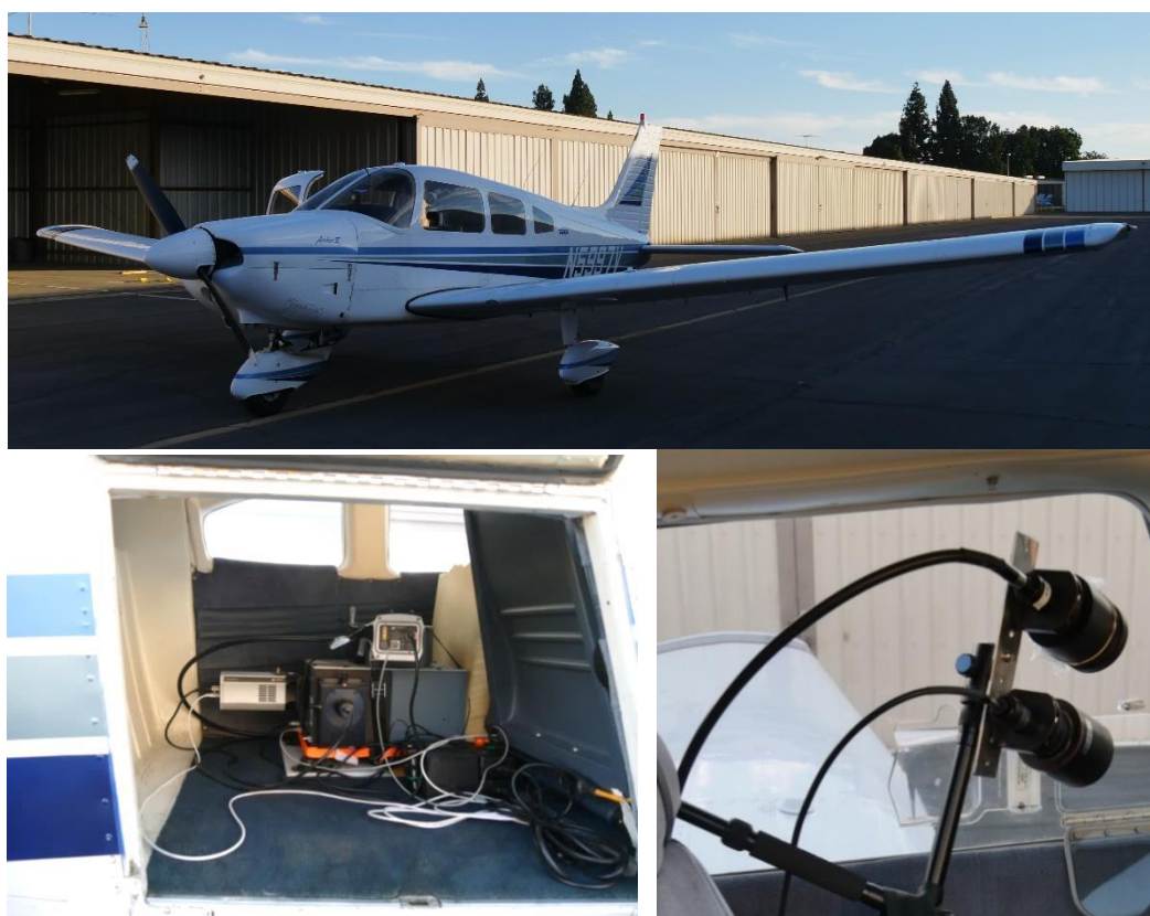
Figure 14. The Piper PA 28 aircraft used for large scale optical measurements. The optical equipment is shown in the bottom left picture while the telescope setup is shown.
