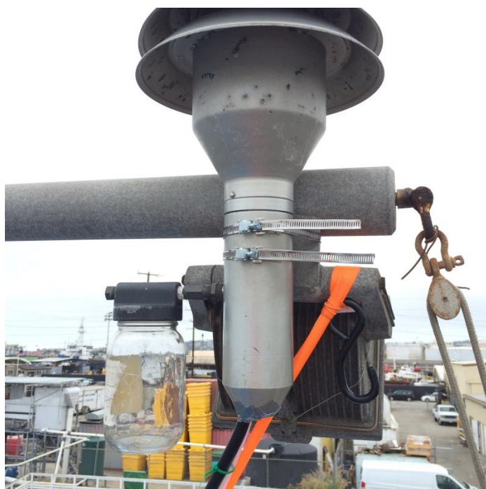
Figure 32. The PM 10 inlet used for gas and particulate sampling. The inlet is made of aluminium and it has been found out later that some of the SO 2 might be adsorbed on its surface.
