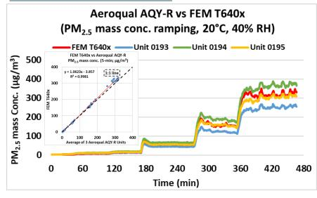
The Aeroqual AQY-R sensors showed very strong correlations with the corresponding FEM PM<sub>2.5</sub> data ( $R^2 > 0.99$ ) at 20°C and 40% RH.
