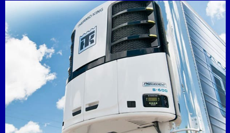
Transport Refrigeration Unit (TRU)
