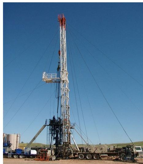
Figure 2.10 – A Workover Rig in Operation
