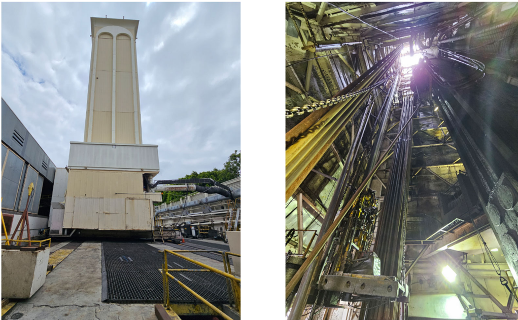
Figure 2.11 – Photo on left shows electrified drilling/workover rig and photo on right shows inside view. Note that this drilling/workover rig is on a rail and can only be used at this specific site
