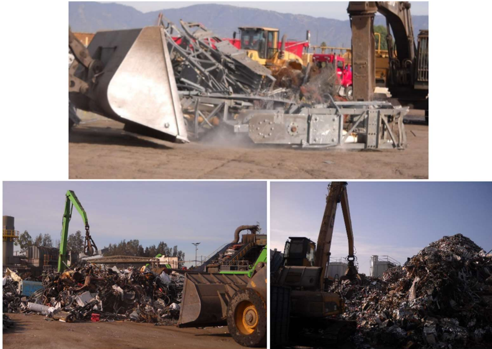
The top image depicts a skip loader. The two bottom images depict grapplers
